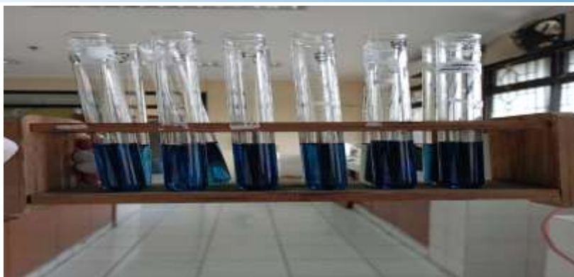
Gambar 1. Pengukuran glukosa sampel minuman metode nelson somogyi
